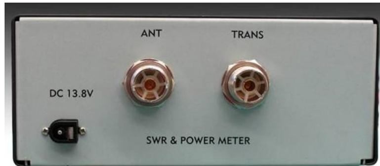
1. Power connector. Note the XCOM SWR meter will operate without power; this only supplies a backlight to the front panel meter gauge
