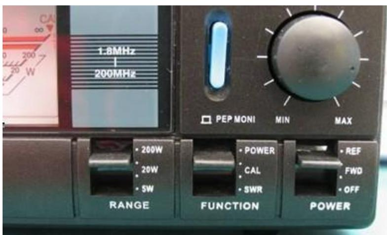
Switch the function switch ⑤ to SWR and note the reading on the top scale of the meter ①.
