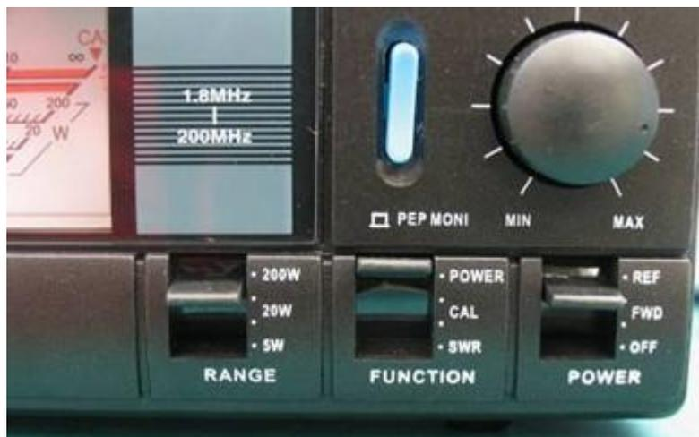
Transmit on the radio and note the reading on the appropriate power scale.
