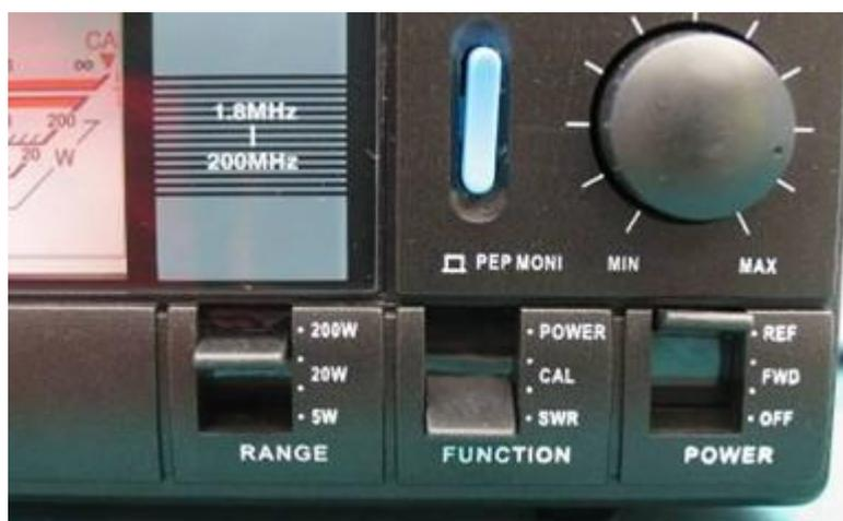
**NOTE:** If the needle ① shows in the red portion of the scale - STOP transmitting immediately. There is a problem with the connections, cables or antenna matching and this could cause damage to the radio.
