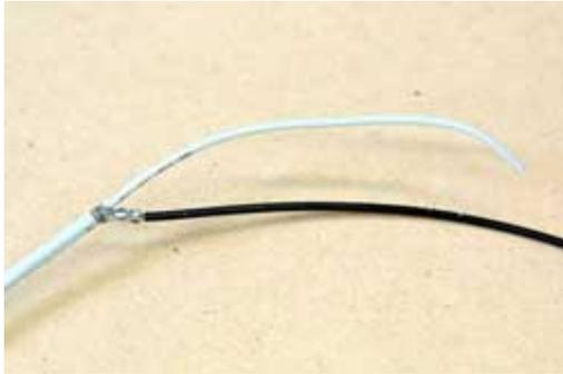
On one end only, trim the shield to around 10mm and attach a piece of black wire about 50mm long
