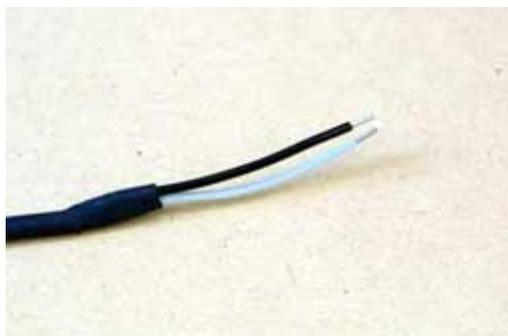
Strip about 40mm from both ends and separate the shield from the cores. On one end only, trim the shield to around 10mm and attach a piece of black wire about 50mm long. Solder and heatshrink over the whole lot. Trim the black wire to the length of the core, strip the shield and pre solder
