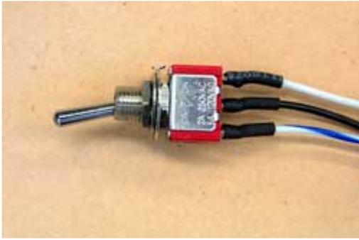
On one end only, trim the shield to around 10mm and attach a piece of black wire about 50mm long. Solder and heatshrink over the whole lot. Trim the black wire to the length of the other cores, strip the shield and solder to the toggle switch
