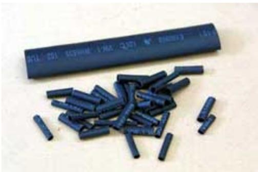
Prepare the Heatshrink for the job. You will need three sizes for the harness - 1.5mm for the individual wires, 3mm for things like the headset jacks and multiple wires and 12 to 15mm for the bundle of wires coming from the DB15 plug.
