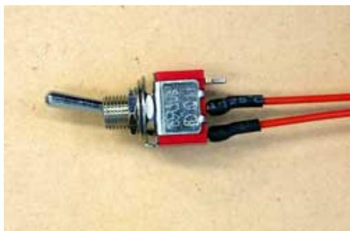
Strip about 40mm from both ends and separate the shield from the cores. On one end only, trim the shield to around 10mm and attach a piece of black wire about 50mm long. Solder and heatshrink over the whole lot. Trim the wire to the length of the core, strip the shield and pre solder. Attach to the toggle switch and heatshrink as shown.
