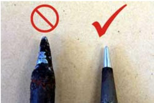
Clear the bench and give yourself lots of room. Now that the bench is clear get your tools ready.... Use a proper soldering iron made for the job. Do not attempt to solder small connections with a large soldering iron because it will not work - you will simply end up with large clumps of poorly connected solder. Use good quality solder and have lots of heatshrink ready.
