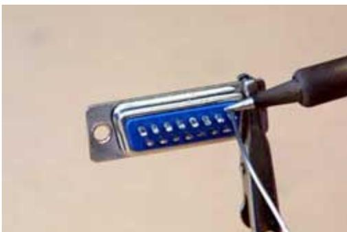
Clamp the DB 15 plug securely and pre solder the pins. The pins are numbered left to right on the back starting top left corner as number 1 and continuing the top row to number 8. The bottom row is 9 to 15.
