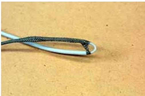
Strip about 40mm from both ends and separate the shield from the cores by separating the mesh and bending the wire through the hole. We use a small screwdriver to assist
